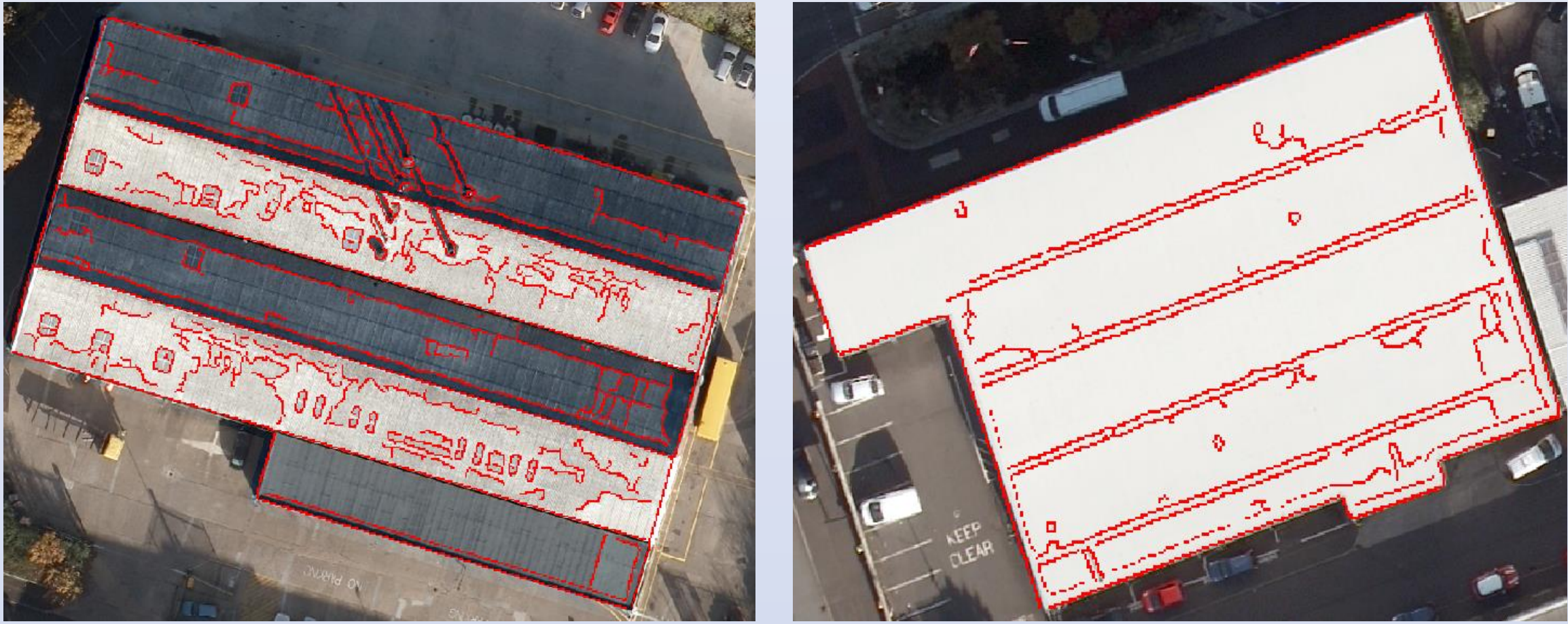
Figure 1. Edge detection results (red) from a. Flat roofed building and b. M-Shaped roofed building overlaid onto the orthophoto
