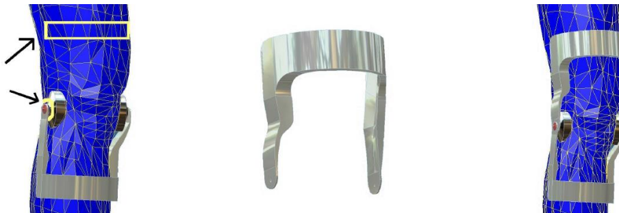
Figure 16: An example of top down design modelling being used to identify key geometry, aiding the design process of a knee brace
