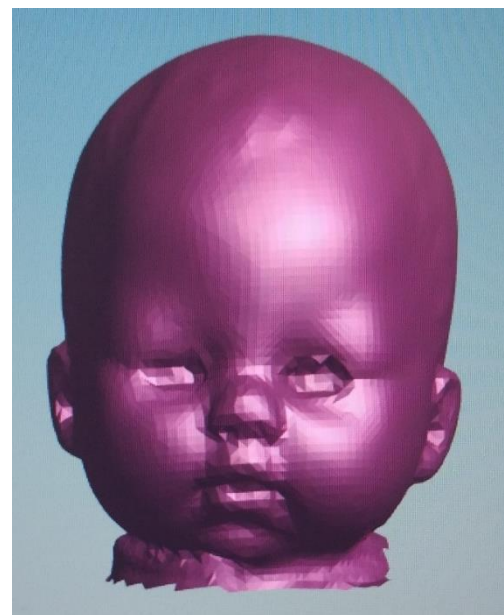
Figure 33: Facial scan data taken from a realistic infant doll for the intent of developing a neonatal CPAP mask
