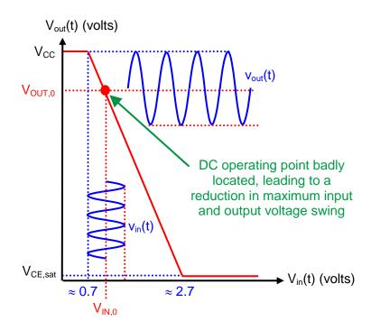
• If the transistor is allowed to enter either the cut-off mode or the saturation mode, the output signal is clipped, and distortion is thus introduced. Our circuit is no longer a linear amplifier.
