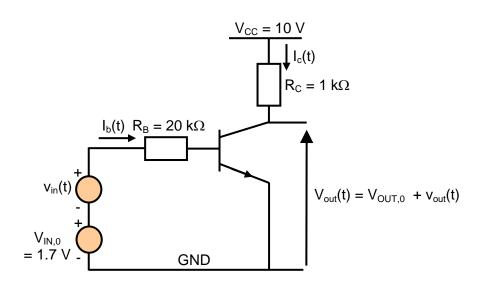
The DC voltages  $V_{IN,0}$  and  $V_{OUT,0}$  are the *bias voltages*. Their values can be chosen by the circuit designer so that the amplifier operates right in the middle of the forward active region. In fact, in
