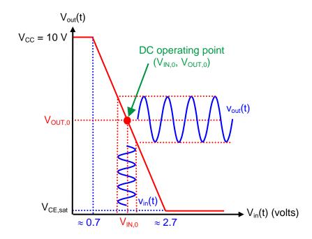
• An ideally located DC operating point (optimal biasing) allows maximal swings for both input and output voltages, as illustrated below.
