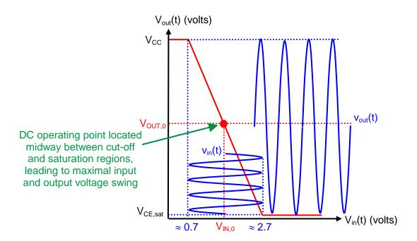
• A badly located DC operating point (non-optimal biasing) can significantly reduce the maximal swings for both input and output voltages, as illustrated below.
