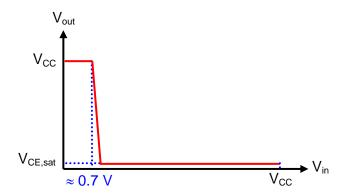
This circuit could be used as a logic inverter (see RTL, DTL, and TTL logic families, aka the saturated bipolar logic families, widely used between the 60s and the 80s).
