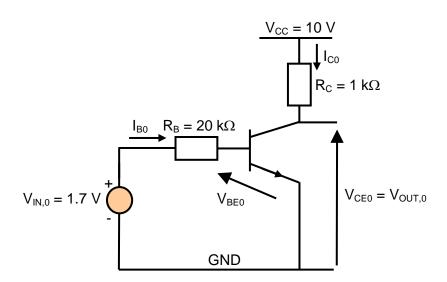
As usual, we assume that the BJT is in the forward active mode (to be checked later). We can write:  $V_{IN,0} \approx R_B I_{B0} + 0.7 \Rightarrow I_{B0} \approx \frac{V_{IN,0} - 0.7}{R_B} \approx 50 \ \mu\text{A}.$
