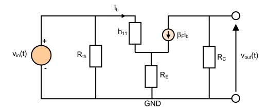
We can show that  $v_{out}(t) = -R_C \beta_F i_b$ .
