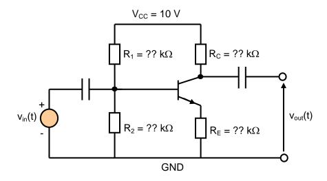
The design issue consists of determining the values of the four resistances  $R_1$ ,  $R_2$ ,  $R_C$  and  $R_E$  so as to meet the specifications. To this end, we must remember several results that have previously been obtained for the common-emitter amplifier with negative feedback.
