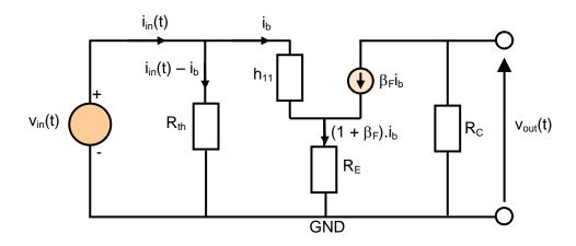
Without feedback (R<sub>E</sub> = 0), we would obtain  $r_{in} = \frac{h_{11}R_{th}}{h_{11}+R_{th}} \approx 1.1$  k $\Omega$ . So, negative feedback has increased the input resistance, which is really good!
