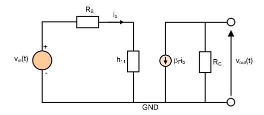
We can show that  $v_{out}(t) = -R_C \beta_F i_b$ . In addition, we can write  $v_{in}(t) = (R_B + h_{11})i_b$ . The small-signal voltage gain of the common-emitter amplifier is thus given by
