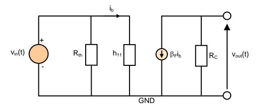
We can show that  $v_{out}(t) = -R_C \, \beta_F \, i_b$ . In addition, we can write  $v_{in}(t) = h_{11} \, i_b$ . The small-signal voltage gain of the common-emitter amplifier is thus given by
