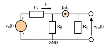
We can show that  $v_{out}(t) = -R_C \beta_F i_b$ .
