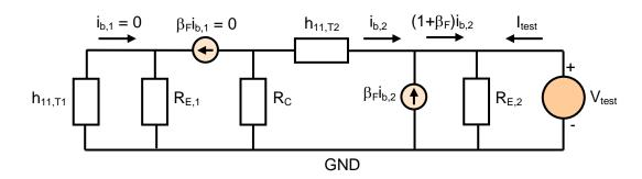
We can write:  $h_{11,T1}i_{b,1}+R_{E,1}\left(1+\beta_F\right)i_{b,1}=0\,,$  which leads to  $i_{b,1}=0\,.$
