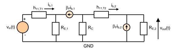
We can show that  $v_{out}\left(t\right) = R_{E,2}\left(1 + \beta_F\right)i_{b,2} \approx R_{E,2}\,\beta_F\,i_{b,2}$  .
