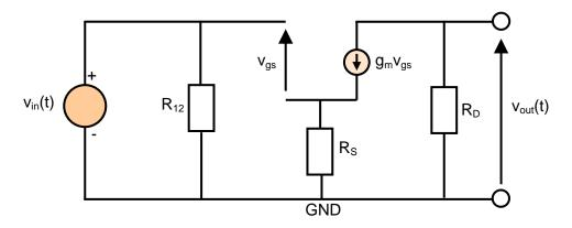
The resistance  $R_{12}$  is given by  $R_{12} = \frac{R_1 R_2}{R_1 + R_2} ~\approx 833 ~k\Omega.$
