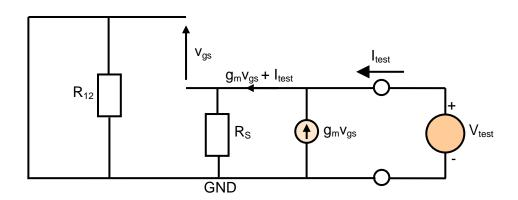
We can write:  $v_{gs} = -g_m R_S v_{gs} - R_S I_{test}$ , which leads to  $v_{gs} = -\frac{R_S}{1 + g_m R_S} I_{test}$ . In addition, we have  $V_{test} = -v_{gs}$ .
