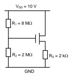
Due to the voltage divider formed by  $R_1$  and  $R_2$ , we can show that the gate voltage  $V_G$  (with respect to ground) is given by  $V_G = \frac{R_2}{R_1 + R_2} V_{DD} = 2 \text{ V}$ . Then, we can write  $V_G = V_{GS0} + R_S I_{D0}$ .
