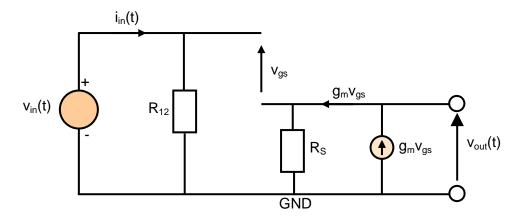
The small-signal output resistance is given by  $r_{out} = \frac{V_{test}}{I_{test}} |_{v_{in}(t) = 0}$ .
