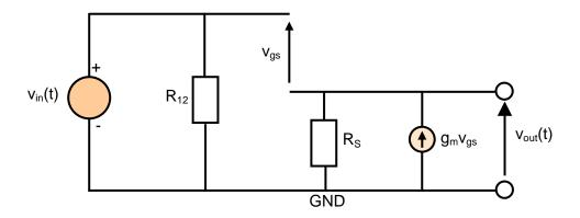
The resistance  $R_{12}$  is given by  $R_{12}=\frac{R_1R_2}{R_1+R_2}$  = 1.6  $M\Omega.$
