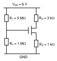
Due to the voltage divider formed by  $R_1$  and  $R_2$ , we can show that the gate voltage  $V_G$  (with respect to ground) is given by  $V_G = \frac{R_2}{R_1 + R_2} V_{DD} = 1$  V. Then, we can write  $V_G = V_{GSO} + R_S I_{DO}$ .
