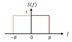
We define the spectrum over the interval [-B, +B] to ensure that the time-domain signal s(t) is going to be a real function. The inverse Fourier transform of S(f) is given by
