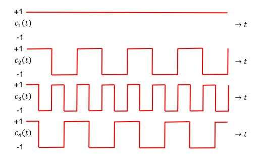
For instance, the notation  $c_1(t)=(+1,+1,+1,+1)$  means that the pattern (+1,+1,+1,+1) is repeated every T second, i.e., for each successive symbol to be transmitted, which implies that the codes are indeed periodic and the duration of one bit in the code is given by  $\frac{T}{N}=\frac{T}{4}$  seconds.
