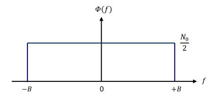
In this case, the total power of the noise process is given by  $P_{total} = \int_{-B}^{+B} \Phi(f) df = N_0 B$ .
