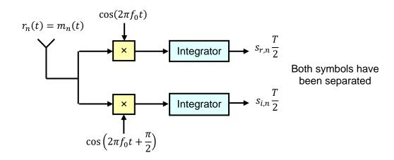
In a similar fashion, to recover the symbol  $s_{i,n}$ , we multiply  $r_n(t) = m_n(t)$  by  $g(t) = \cos\left(2\pi f_0 t + \frac{\pi}{2}\right)$  and then integrate the result as follows:  $\int_{n \cdot T}^{(n+1) \cdot T} m_n(t) \cdot g(t) dt = s_{r,n} \cdot \int_{n \cdot T}^{(n+1) \cdot T} \cos(2\pi f_0 t) \cdot \cos\left(2\pi f_0 t + \frac{\pi}{2}\right) dt + s_{i,n} \cdot \int_{n \cdot T}^{(n+1) \cdot T} \cos^2\left(2\pi f_0 t + \frac{\pi}{2}\right) dt = s_{i,n} \cdot \frac{T}{2}.$
