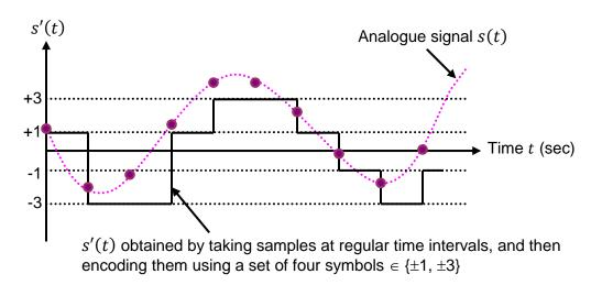
The digital signal s'(t) can be seen as a vector of 4-ary real symbols  $s_n \in \{-3, -1, +1, +3\}$ ,  $n \in \{0, 1, 2, 3, ...\}$ . A particular symbol  $s_n$  is obtained by quantizing the sample s'(nT), where T denotes the sampling period. Since the number of values taken by symbols  $s_n$  is finite, these symbols are said to be discrete.
