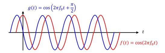
The functions f(t) and g(t) are orthogonal since  $\int_{t_0}^{t_0+T} f(t) \cdot g(t) dt = \int_{t_0}^{t_0+T} \cos(2\pi f_0 t) \cdot \cos\left(2\pi f_0 t + \frac{\pi}{2}\right) dt = \frac{1}{2} \int_{t_0}^{t_0+T} \cos\left(4\pi f_0 t + \frac{\pi}{2}\right) dt + \frac{1}{2} \int_{t_0}^{t_0+T} \cos\left(\frac{\pi}{2}\right) dt = 0.$
