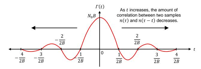
Remarkably, this expression indicates that, if the time t between two samples  $n(\tau)$  and  $n(\tau-t)$  is a multiple of  $\frac{1}{2B}$ , then these samples are not correlated. Therefore, if we were to sample such noise process every  $\frac{1}{2B}$  seconds, then this noise would appear as if it was perfectly white.
