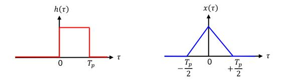
In this example, y(t)=0 for  $t<-\frac{T_p}{2}$  or  $t>\frac{3T_p}{2}$ . y(t) is maximal for  $t=\frac{T_p}{2}$ .
