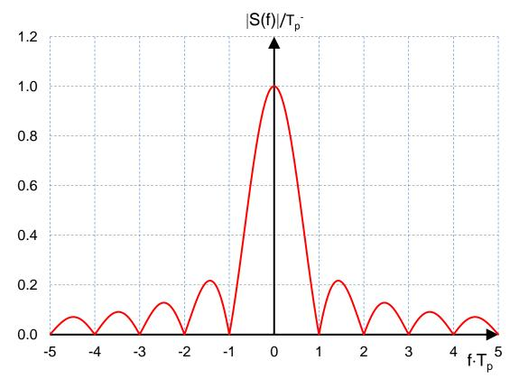
Strictly speaking, the bandwidth of the square pulse is infinite. This means that, if one attempts to transmit such pulse through a practical communication system, some (high) frequency components will be filtered out, which will result in distortion in the time-domain.
