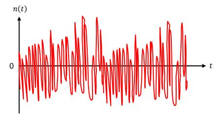
A pure white noise process cannot exist in the real world, but a noise process can still be considered as white in practice if its PSD is constant in the bandwidth of interest. In other words, if no signal in our communication system contains frequency components outside a band
