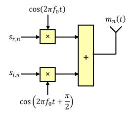
At the receiver side, we can separate the symbols  $s_{r,n}$  and  $s_{i,n}$  by exploiting the orthogonality of the functions  $f(t) = \cos(2\pi f_0 t)$  and  $g(t) = \cos\left(2\pi f_0 t + \frac{\pi}{2}\right)$ .
