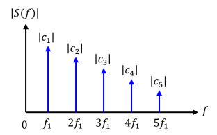
This discrete spectrum shows the distribution of the signal energy on the frequency axis.
