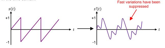
The bandwidth of a signal is defined as the frequency band occupied by its spectrum. Depending on their shape in the time domain, certain types of signals have a finite bandwidth (typically, signals with smooth variations, e.g., sine waves), while some others have an infinite bandwidth (typically, signals with infinitely sharp variations, e.g., square waves). Bandwidth is
