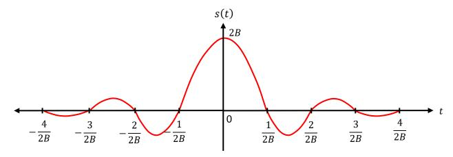
The shape of this sine cardinal pulse is very smooth, which explains why its bandwidth is not infinite, unlike the square pulse studied previously. It can be seen that, when the bandwidth *B* is decreased, the sine cardinal pulse "spreads out", i.e., becomes even smoother.
