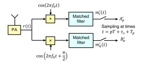
Assuming, for simplicity's sake, that the delay  $\tau_0$  corresponds to the fastest path whereas the delay  $\tau_{L-1}$  is associated with the slowest path, we typically have  $\tau_0 \le \tau_S \le \tau_{L-1}$  because it makes sense to sample the baseband signal any time after the arrival of the fastest path and before that of the slowest path.
