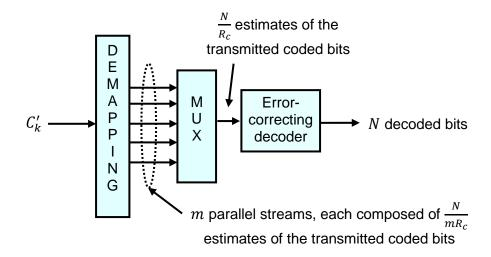
At this stage, we can compute the bit error rate (BER) which is a measure of the bit error probability  $P_{eb}$ . To do so, the sequence of information bits is compared with the decoded sequence: an error event is counted every time a decoded bit is different from the corresponding transmitted information bit. Finally, the BER is obtained by dividing the total number of errors by the number N of transmitted information bits.
