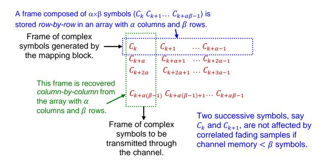
If a multipath channel changes very slowly, then the 2-D array used for interleaving needs to be very large to guarantee independence between received samples. Hence, the use of interleaving may not be a practical option in some applications for which the transmission delay or frame size are limited.
