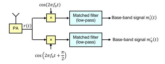
At the quadrature matched filter output, we obtain the base-band signal  $m'_a(t)$  given by
