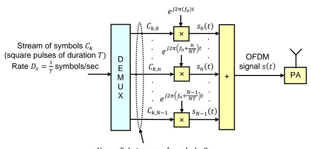
N parallel streams of symbols  $C_{k,n}$  (square pulses of duration NT) Symbol rate  $D_{s,n} = \frac{1}{NT}$  symbols/sec Note that, in the figure above, the notation
