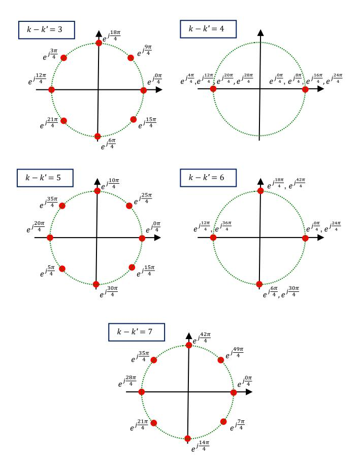
After demodulation, i.e., removal of the term  $e^{j(2\pi f_0t)}$  from the received signal, the receiver can recover all symbols  $\mathcal{C}_k$  by performing a discrete Fourier transform (DFT) of the channel estimates representing the N symbols  $\bar{\mathcal{C}}_p, p \in \{0, \dots, N-1\}$ .
