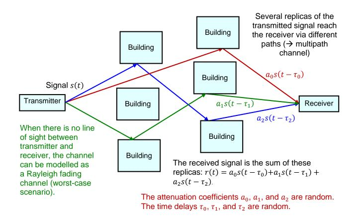
Obviously, we are more particularly worried about the destructive nature of the interference since its detrimental effect can sometimes make the signal completely undetectable by the receive antenna.
