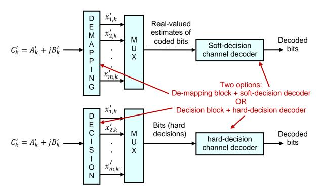
The "de-mapping block + soft-decision decoder" option has much better error-correction capabilities than the "decision block + hard-decision decoder"
