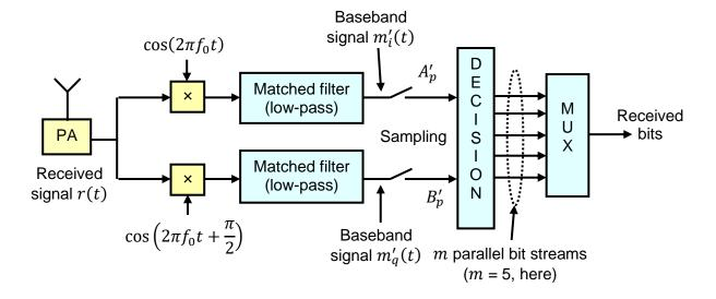
The received signal must be amplified since the signal power received by the antenna is usually quite low.
