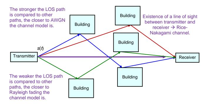
When there is a line of sight between transmitter and receiver, we have  $E\{w_{p,1}\}=m\neq 0$  and  $E\{w_{p,2}\}=0$ . In this case, the fading sample  $h_p$  follows a Rice-Nakagami distribution given by
