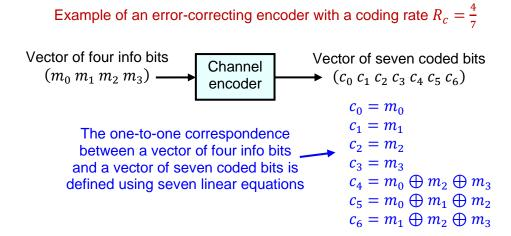
There are  $2^4 = 16$  possible vectors of info bits. Thus, only 16 vectors of coded bits can be generated among the  $2^7 = 128$  possible ones  $\rightarrow$  Only 16 specific binary sequences can exist at the encoder output. This knowledge can be exploited at the receiver side to correct transmission errors.
