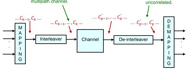
The interleaving technique consists of *scrambling* the sequence of successive symbols before transmitting it. If the size of the interleaving function is sufficiently large, then two successive symbols, say  $C_{k-1}$  and  $C_k$ , can in fact be transmitted at very different times and thus be affected by independent fading samples despite the inherent memory of the channel.
