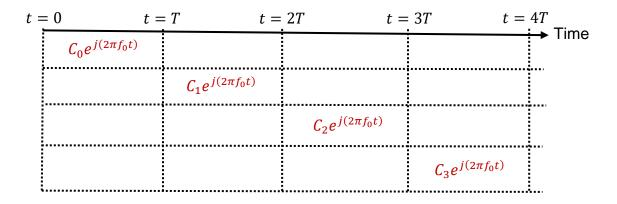
In an OFDM communication system, the expression of the modulated signal generated by the transmitter between t = kT and t = (k + 1)T is given by
