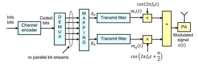
The channel encoding process basically consists of introducing some clever dependency between transmitted bits: the value of any coded bit depends on the values of the preceding and succeeding coded bits. In other words, with channel coding, only some specific binary sequences can be transmitted, whereas other sequences are forbidden. When this technique
