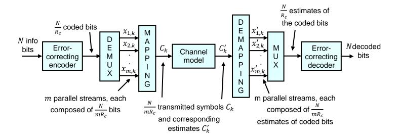
Then, the transmission of constellation symbols  $C_k = A_k + jB_k$  over the channel is simulated by computing the channel outputs  $A'_k$  and  $B'_k$  as a function of  $A_k$  and  $B_k$ .
