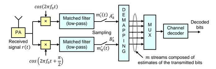
At the receiver side, an estimate  $C'_k = A'_k + jB'_k$  of the corresponding transmitted complex symbol  $C_k$  is available, at each time kT, at the sampling device output.
