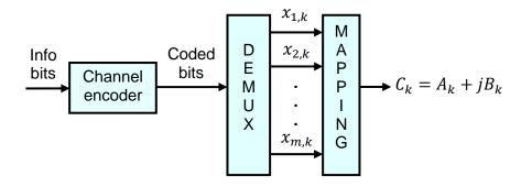
The mapping operation converts this m-bit vector  $(x_{1,k}, x_{2,k}, ..., x_{m,k})$  into a pair of real-valued symbols  $A_k$  and  $B_k$ , or equivalently a complex symbol  $C_k = A_k + jB_k$  that can take  $M = 2^m$  different values. Traditionally, we employ Gray mapping since such labeling technique minimizes the bit error probability for a given symbol error probability.
