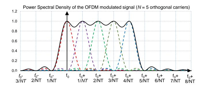
We notice that there is a significant overlap of the individual spectra  $S_n(f)$ . The overall spectrum of the combined OFDM signal s(t) can be seen as ranging, approximately, from  $f_0 - \frac{1}{NT}$  to  $f_0 + \frac{N-1}{NT} + \frac{1}{NT}$ . Therefore, the bandwidth required for the transmission of this signal is
