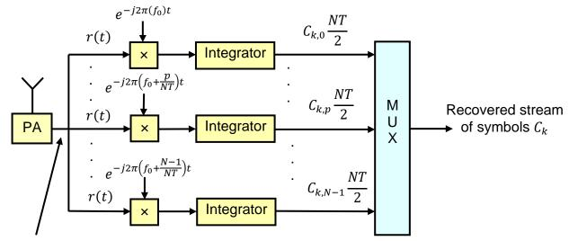
Received OFDM signal r(t)Here, we assume a noiseless channel for which r(t) = s(t)
