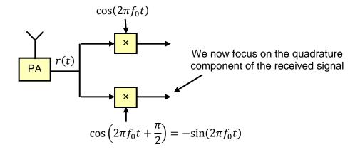
To obtain the base-band signal  $m_q'(t)$ , which is an estimate of the base-band signal  $m_q(t)$ , present at the transmitter side, one has first to demodulate the signal r(t) by mixing it with a locally-generated carrier signal  $\cos\left(2\pi f_0 t + \frac{\pi}{2}\right) = -\sin(2\pi f_0 t)$ .
