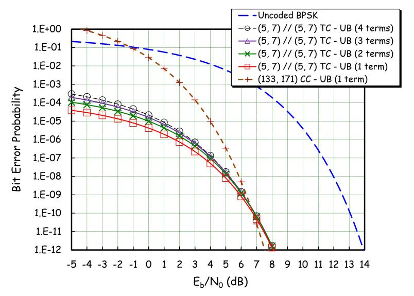
Comparison between union bound and simulation results the union bound of a turbo code is not quite as tight as it is for a CC. Due to the non-ML decoding of turbo codes?
