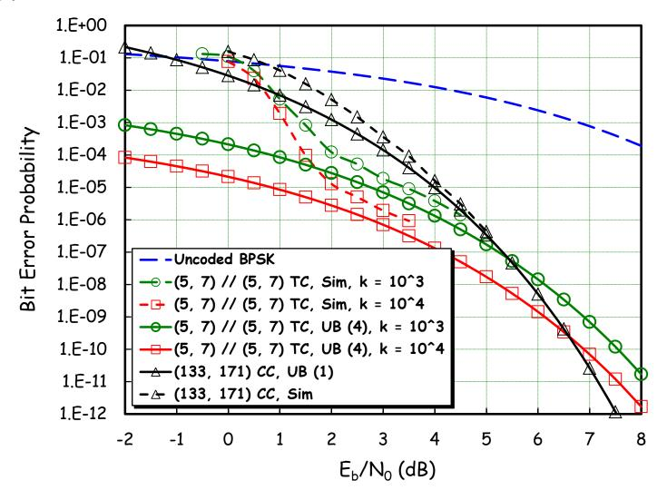
Comparison between several rate-1/3 turbo codes built using different RSC codes, for k = 1000. Best results obtained with 8- and 16-state RSC codes.
