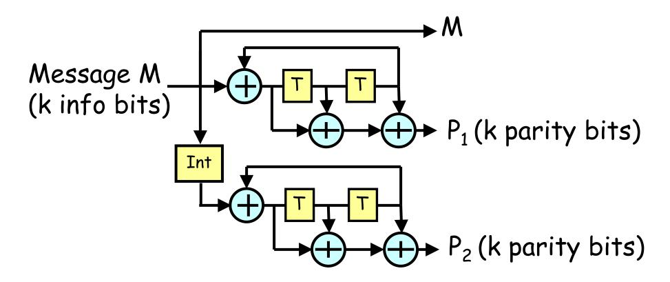
The codeword  $C \equiv M + P_1 + P_2$  is composed of k info bits and 2k parity bits.
