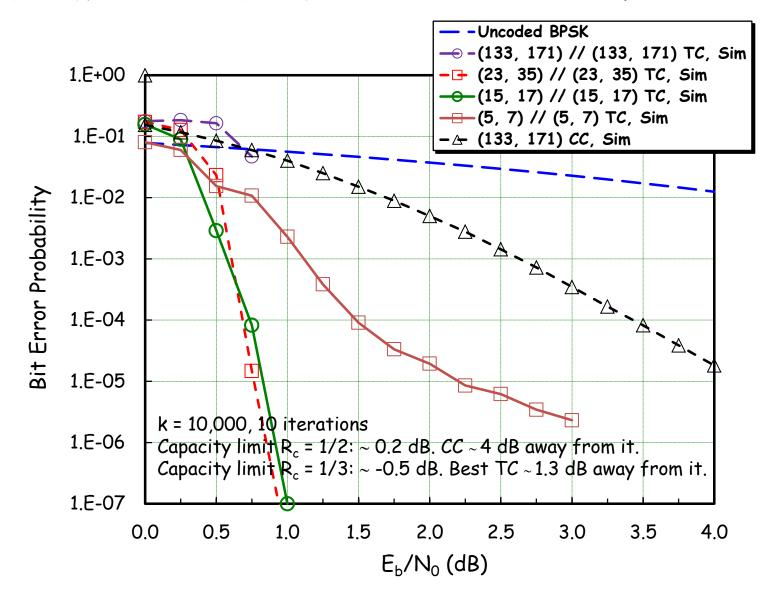
Error performance is improved by increasing the number of decoding iterations, but there is no real need to use more than 5-10 iterations in practice.
