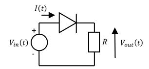
Study the operation of this circuit by using the laws of circuit theory (here, Kirchhoff's voltage law and Ohm's law) and the two-state model for a diode.
