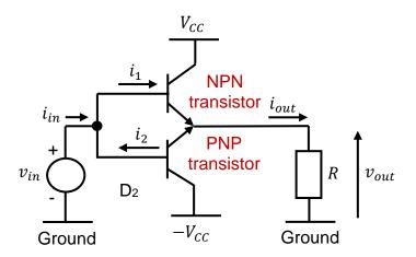
Note that a BJT can be modelled using a diode and a dependent current source only if this BJT does not saturate. This condition is satisfied in this circuit.
