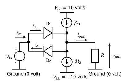
This circuit is designed using two diodes  $D_1$  and  $D_2$ , each of them having a threshold voltage  $V_d$ , a resistance R, and two dependent current sources  $\beta i_1$  and  $\beta i_2$ , where  $\beta$  is a constant parameter equal to 100, and  $i_1$  and  $i_2$  are the currents flowing through diodes  $D_1$  and  $D_2$ , respectively.
