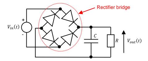
Study the operation of the circuit assuming that the input signal  $V_{in}(t)$  is a sinusoidal signal.
