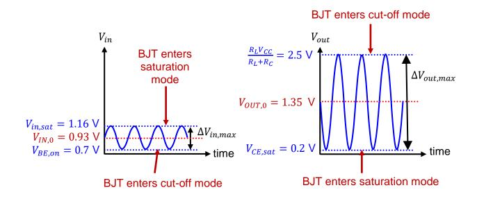
The optimal value of  $V_{IN,0}$  is located midway between the start of the cut-off region, corresponding to  $V_{in} = V_{BE,on}$ , and the start of the saturation region, corresponding to  $V_{in} = V_{in,sat}$ :
