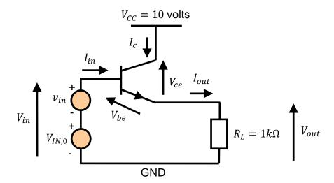
The input voltage  $V_{in}$  is now composed of two voltage sources  $V_{IN,0}$  and  $v_{in}$  connected in series. Hence, we can write  $V_{in} = V_{IN,0} + v_{in}$ .
