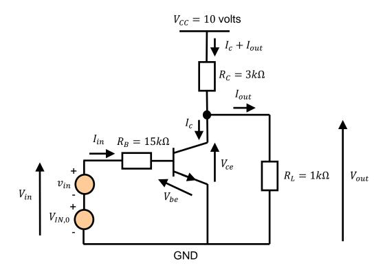
The input voltage  $V_{in}$  is now composed of two voltage sources  $V_{IN,0}$  and  $v_{in}$  connected in series. Hence, we can write  $V_{in} = V_{IN,0} + v_{in}$ .
