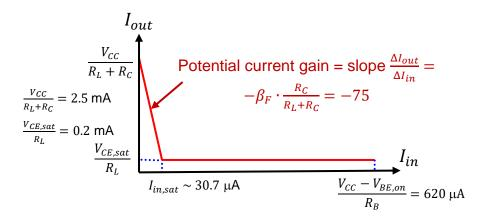
We can observe the potential of the common-emitter circuit as a current amplifier when the BJT is forward active because, in that mode, the output current  $I_{out}$  is a linear function of the input current  $I_{in}$ :  $I_{out} = \frac{1}{R_I + R_C} \cdot [V_{CC} - \beta_F \cdot R_C \cdot I_{in}]$ .
