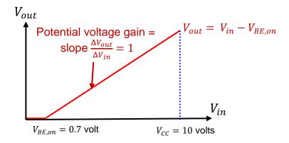
It is observed that the common-collector circuit does NOT have the potential to be a voltage amplifier because the slope  $\frac{\Delta V_{out}}{\Delta V_{in}}$  of the DC voltage transfer characteristic in the forward-active region is only equal to the unit.
