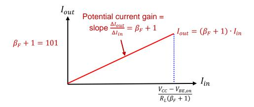
We observe the potential of the common-collector circuit as a current amplifier because, in the forward-active region, the output current  $I_{out}$  is a linear function of the input current  $I_{in}$ :
