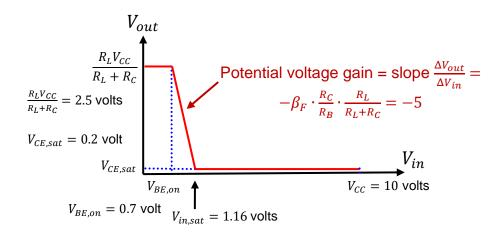
The voltage  $V_{in,sat}$  corresponds to the value of the input voltage at which the BJT leaves the forward-active mode to enter the saturation mode.
