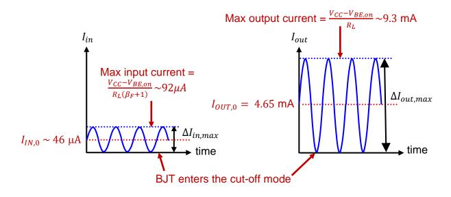
The maximum value for the maximum output current swing,  $\Delta I_{out,max}$ , is given by  $\frac{V_{CC}-V_{BE,on}}{R_L}\sim 93$  mA.
