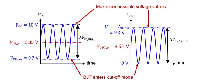
The optimal value of  $V_{IN,0}$  is located midway between the start of the cut-off region, corresponding to  $V_{in} = V_{BE,on}$ , and the maximum input voltage in the circuit, corresponding to  $V_{in} = V_{CC}$ :
