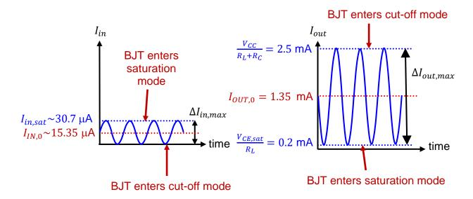
The maximum value for the maximum input current swing,  $\Delta I_{in,max}$ , is given by  $I_{in,sat} \sim 30.7 \, \mu A$ . In other words, the maximum peak-to-peak amplitude of the AC input current,  $i_{in}$ , that guarantees no distortion in  $i_{out}$  cannot exceed  $30.7 \, \mu A$ .
