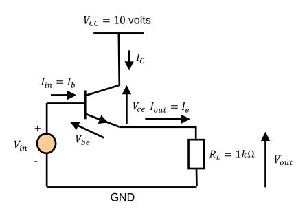
The presence of a load resistance  $R_L$  accounts for the fact that in practice any electronic circuit has its output connected to the input of another downstream circuit, the latter being modelled using a load resistance.
