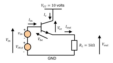
This type of amplifier is referred to as a common-collector amplifier as both input and output ports have the collector as a common reference.
