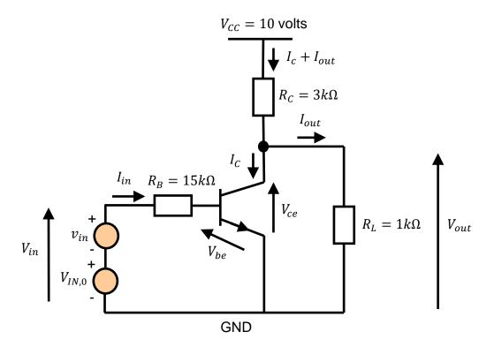
This type of amplifier is referred to as a common-emitter amplifier as both input and output ports have the emitter as a common reference.
