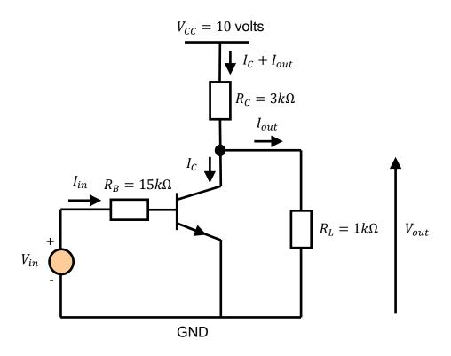
The presence of this load resistance accounts for the fact that in practice any electronic circuit has its output connected to the input of another downstream circuit, the latter being modelled using a load resistance. Also, the fact that there is now a load resistance allows us to introduce the concepts of DC current transfer characteristic, current amplifier, current gain, and so on.
