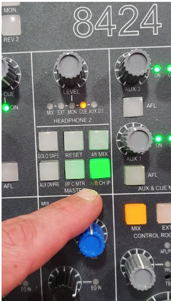
INPUT CHANNEL A : The buttons will turn **GREEN**, indicating the desk channels will receive audio from Pro Tools.
