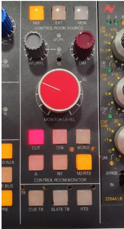
When the Neve 8424 is initialised, the output will be **CUT** to prevent accidental damage to monitor speakers. Press the **CUT** button to unmute.
