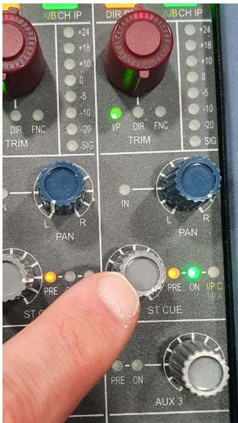
**Using STEREO CUE from the desk.** If you are monitoring channels through the desk, it is possible to send a Cue Mix using the ST CUE pots. By default, these are PRE-FADER. The send just needs to be activated by pressing the ST CUE pot until the green LED shows **ON** (see picture, left)
